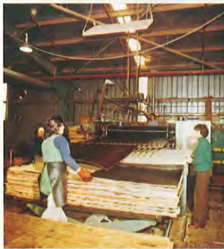
Centre-laying glued veneer for the manufacture of plywood
