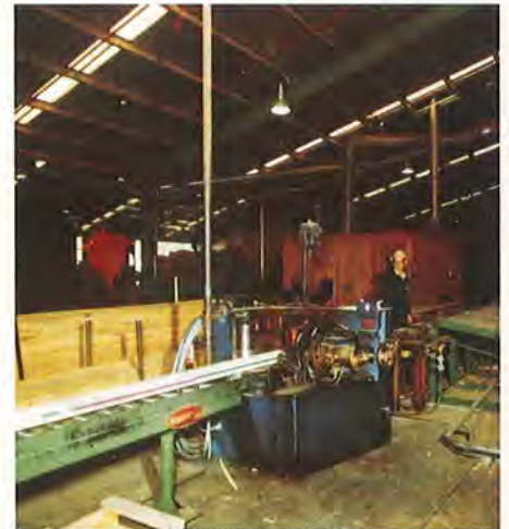
This stress grader colour codes the strength of timber
