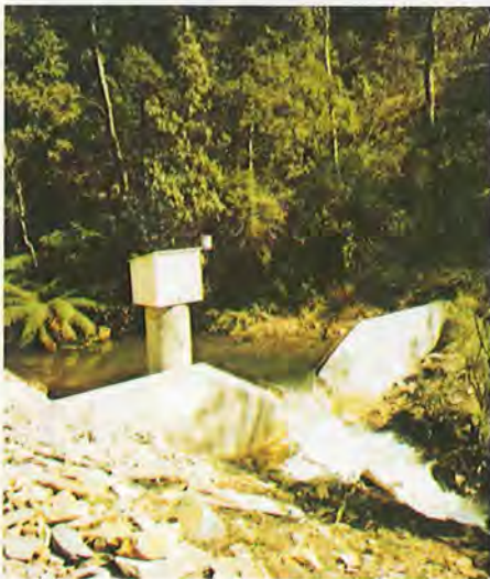
This stream gauging station in the Cotter catchment measures the run-off volume of water
