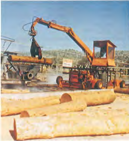
A log is lowered into a steaming hot water vat to make peeling easier for the veneer lathe
